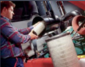
The effective new air filter is easily accessible, and cartridges are simple to replace.
