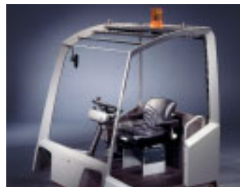
Open safety cage that can be fitted with windows and doors, even after delivery.
