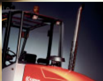
The air filter is totally concealed under the cab, and the exhaust pipe is positioned for minimum interference.
