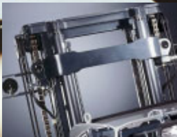
The cross-head in the mast has been made narrower – yet still as strong – for better forward visibility.
