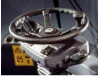
The steering wheel is vertically and horizontally adjustable.
